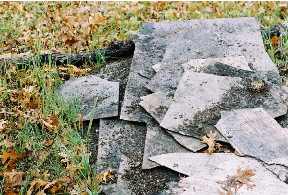
5/12/06 Photo of Pile of Friable Asbestos Debris
