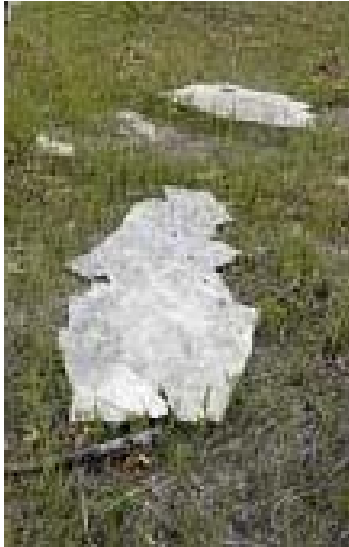
Figure 9 - Large pieces of asbestos debris photographed in mid-May after being exposed on the ground surface by a field burn that was conducted by the IDNR.
