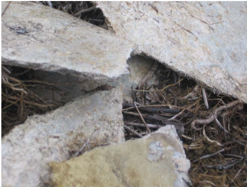
Figure 2 – Close-up of Broken, Weather, and Burned Asbestos Debris near Kellogg Creek These Materials are Friable and Regulated.
