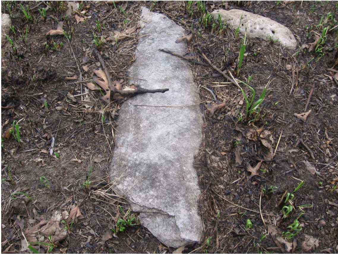
Figure 3 - Large Pieces of Friable Asbestos heave through the ground where weather and fire release toxic fibers
